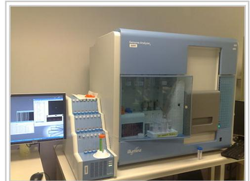
Illumina Genome Analyzer II System. Illumina technologies have set the standard for high throughput massively parallel sequencing.<sup>[46]</sup>
